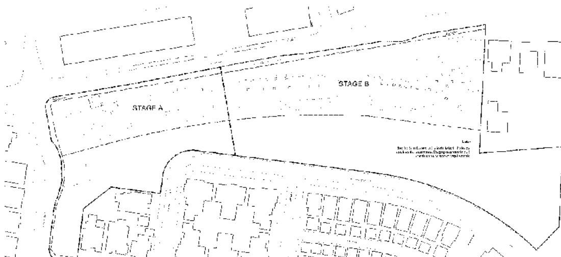
Figure 2: Indicative staging plan showing works divided into Buildings A & B with part of the community lot landscape works with a separate stage for buildings C & D with the remainder of the community lot landscape works.
